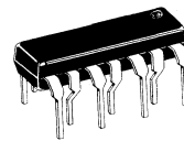
PQ SUFFIX PLASTIC PACKAGE CASE 647
